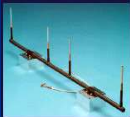
MIP electric antenna, 1m long, including two transmitting and two receiving electrodes (J. G. Trotignon)
