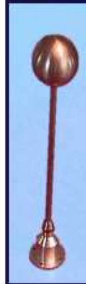
LAP spherical Langmuir probe, 5cm in diameter, made of titanium (R. Boström)
