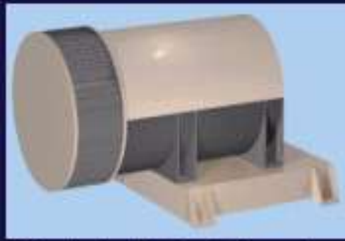
ICA spherical electrostatic analyser with a magnetic mass analyser (R. Lundin)
